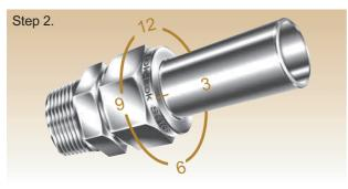
Scribe the nut at the 6 o'clock position and wrench-tighten the nut 1 1/4 turns to the 9 o'clock position, holding the body with a back up wrench.
